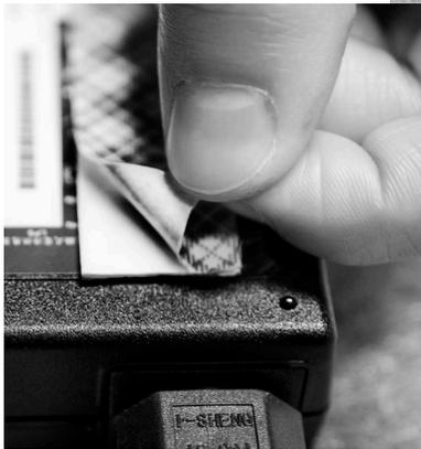
Once positioned to your liking, **PRESS FIRMLY** so the tape adheres properly to **C**. Position the bound length of cable to the left of **the power block** so it will be tucked away under the **WandaNEXT wall-mount Backplate (H)** once it is attached. See the image on the left for a reference.
