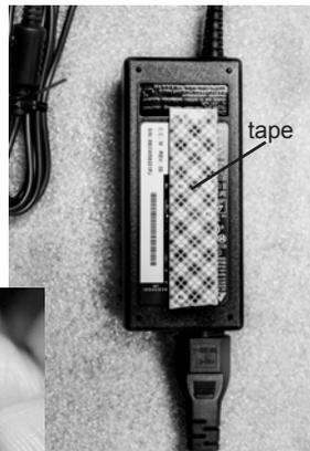
Once removed, position **the power block** on the right side of the back of **C**.
